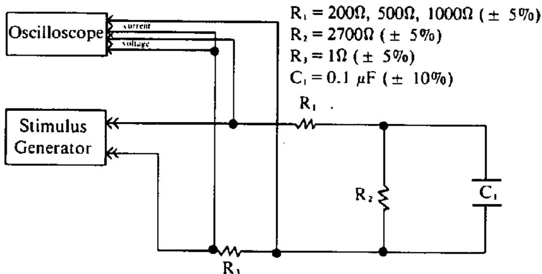
R2 and C1 represent the skin interface and R1 is the electrode pair. Two limits were cited in (1) where 200 ohm represented a lower impedance electrode pair and 500 ohms represents a higher impedance electrode pair of a 5cmx5cm. Note that these impedances represent 2 electrodes in series, hence the single electrode impedance is half of these limits (100 and 250 ohms respectively). Note that this assumes the electrode pair behaves as a linear resistor.
